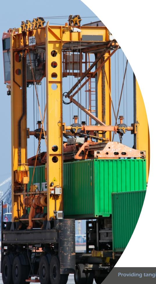
The LCM Systems container weighing system has been designed to be easily retrofitted into the spreader or headerblock of straddle carriers, container cranes and telehandlers. It can be tailored to meet the needs of the individual port, with the standard package being a stand alone system, but with options for a system that is fully integrated into existing terminal operating systems (TOS).
